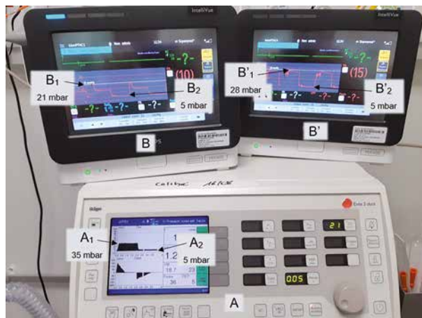
FIGURE 1. Pressure monitoring of our concept showing two different specific pressures in circuits with a single ventilator. We can observe on the single ICU-ventilator screen (A) that the inspiratory pressure is set at 35 mbar (A1) and the expiratory pressure is set at 5 mbar (A2). On the screen of the left monitor, we can observe the pressure in circuit B (B) with an upper pressure (B1 = 21 mbar) regulated with specific pressure regulator of circuit B, and a lower pressure equal to the expiratory pressure set on the ventilator (B2 = 5 mbar). On the screen of the right monitor, we can observe the pressure in circuit B' (B') with a different upper pressure (B'1 = 28 mbar) regulated with another pressure regulator on circuit B', with the same lower pressure (B'2 = 5 mbar)
