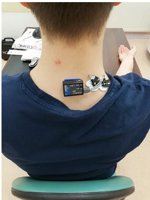
Figure 4. Electrodes and wireless sensors for the descending part of the trapezius muscle.
