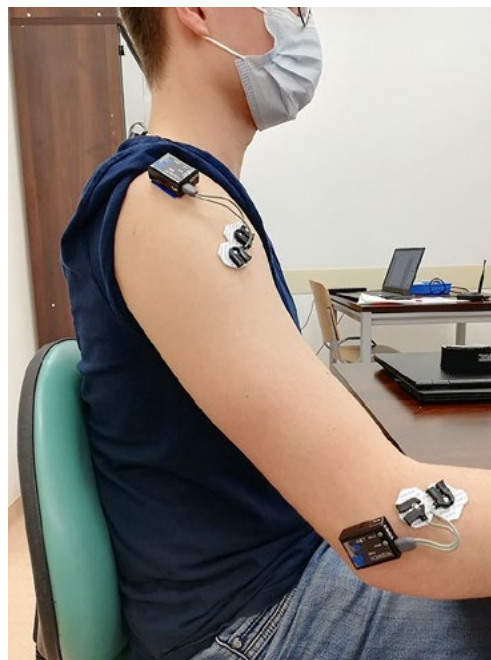
Figure 5. Electrodes and sensors for the anterior part of the deltoid muscle and the wrist radial extensor muscle.
