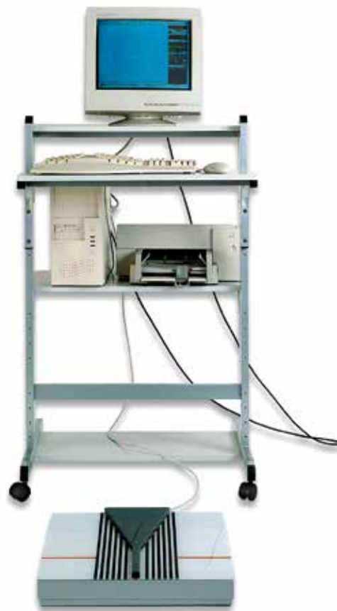
Figure 1. The apparatus for the test by moiré method [11]
