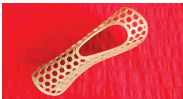
Fig. 7. Orthosis 3D printed by Fucco [116] © H. Dodziuk
