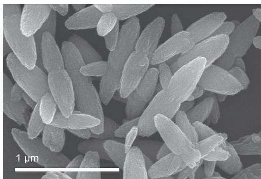
**Fig. 3.** SEM image of the peanut-like ZnO particles synthesized in gelatin matrix (Gan et al., 2010, with permission from Yong Gan et al., Copyright © 2010)
