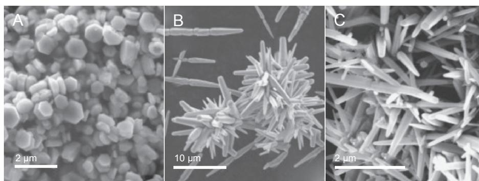
**Fig. 7.** SEM micrographs of ZnO crystals obtained by biomineralization using ZnO-binding peptide: A) using 0.5 mg/ml ZnO-binding peptide + equimolar concentrations of  $\text{Zn}(\text{NO}_3)_2$  and urotropin; B) equimolar concentrations of  $\text{Zn}(\text{NO}_3)_2$  and urotropin (no peptide); C) control reaction containing 0.5 mg/ml of bovine serum albumin (Tomczak et al., 2009 with permission from Elsevier, Copyright © 2008)
