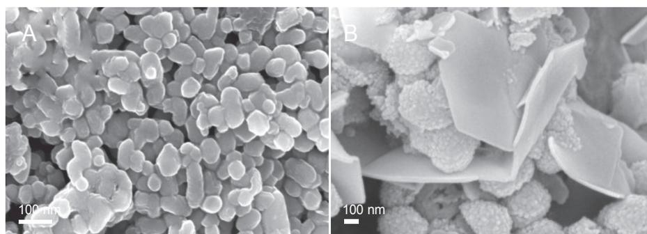
**Fig. 5.** Field-emission SEM micrographs showing: A) raspberry- and plate-like ZnO structures synthesized using *Bacillus cereus* as biotemplate (Hussein, 2009, with permission from Elsevier, Copyright © 2009); B) ZnO nanostructures synthesized using *Aeromonas hydrophila* as biotemplate (Jayaseelan et al., 2012 with permission from Elsevier, Copyright © 2012)
