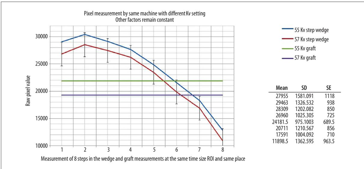
**Figure 7.** Illustrates the pixel value measurement for 8 steps from the step wedge using different exposure factors in the same machine using automatic exposure control. An average variation of 7.6% (5.2 to 14.9) in the pixel values was observed. A variation of 11% was observed in the pixel values of graft. Mean/Standard Deviation (SD) and Standard Error (SE) for step wedge given.
