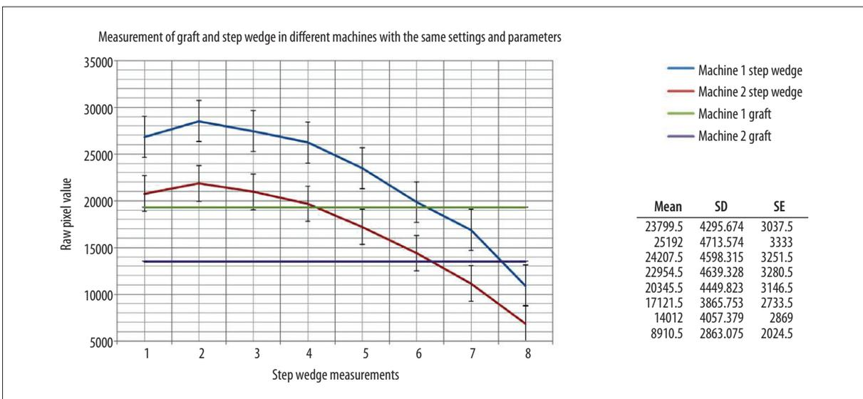
**Figure 8.** Illustrates the pixel value measurement for 8 steps from the step wedge using same exposure factors with different machines. An average variation of 27.5% (22.6 to 37) in the pixel values was observed. A variation of 30% was observed in the pixel values of graft. Mean/Standard Deviation (SD) and Standard Error (SE) for step wedge given.
